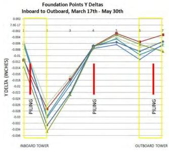
Figure 2. Foundation Settling, Inboard to Outboard
