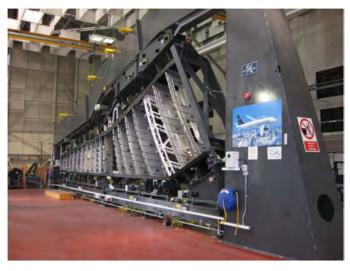
Figure 1. C-Series Demonstrator Wing Box Jig, Belfast
