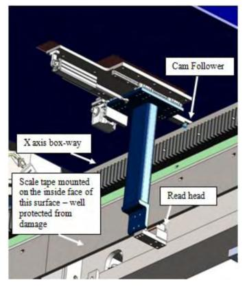
Figure 7. Diagram showing the read head mounting, and rail follower.
