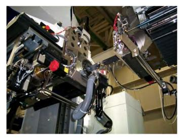
Figure 2. Fastening heads of the ASAT2 machine.
