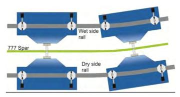
Figure 5. Dry and wet carriage transition through the spar inflection.
