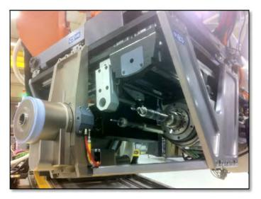
Figure 4. Multi-function end effector. Left to right: nose piece, camera, hole probe, spindle
