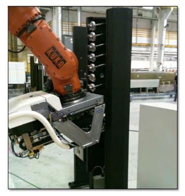
Figure 7. Coupon stand and tool change station
