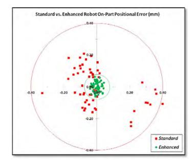
Figure 3. Accuracy comparison: Standard vs. Enhanced
