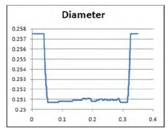
Figure 8. Hole profile data collected by probe
