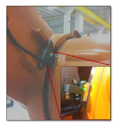
Figure 2. Secondary encoder mounted to output of robot axis
