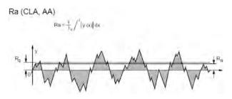
Figure 1. Calculation of average surface roughness (Ra) per ISO 25178-2.
