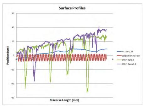
Figure 4. Surface profile of CFRP drilled hole.
