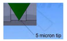
Figure 2. Five micron probe tip shown with 0.25 mm ply thickness and 25 micron deep tear out.
