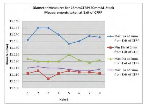
Figure 8. Axial location affects diameter measurements.
