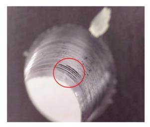
Figure 12. Surface finish defects in under-sized drilled hole
