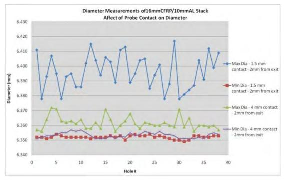
Figure 7. Hole probe diameter size effects.
