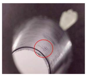
Figure 13. Surface finish defects in reamed hole.
