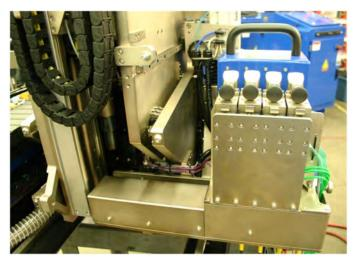
Figure 5. Four Cartridge banks ready to release bolt
