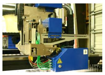
Figure 2. Bolt Cartridges loaded
