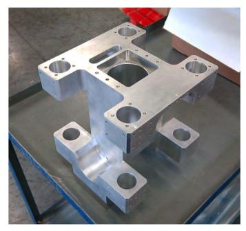
Figure 3. Spindle housing
