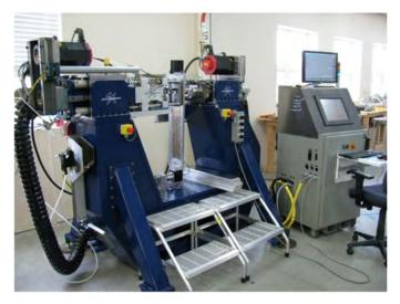
Figure 1. Automated squeeze riveting machine utilizing the coaxial head design
