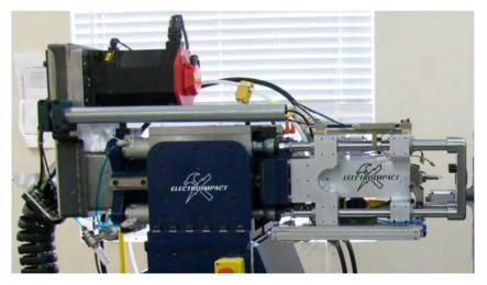
Figure 2. Coaxial riveting head
