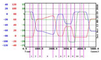
Figure 13. Plot from CNC showing axis positions during a full cycle
