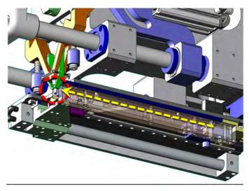
Figure 10. Rivet injector showing feed path and rivet being snapped into fingers (circled)
