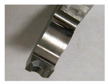
Figure 9. NAS1097\*\*6 rivet finger tip detail
