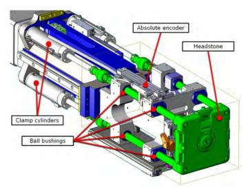
Figure 4. Floating headstone assembly
