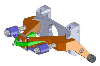
Figure 6. Driver and pressure pad, ready to insert rivet ("drive" position)
