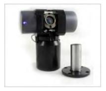
Figure 7. The Active Target is a tool that should not be overlooked when compensating very large machine tools.
