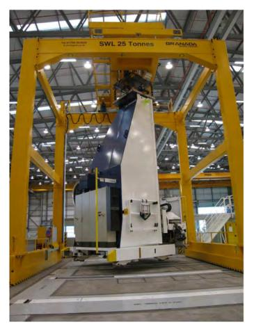
Figure 2. This 5 axis moving column wing fastening machine has a working envelope far exceeding the operators reach.
