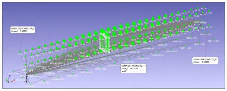
Figure 13. Uncertainty analysis of the previous cell, using a tracker station at each end of the cell. Error is now reasonable at both ends but unacceptable in the center.
