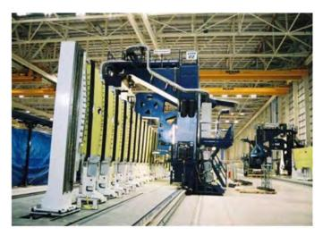
Figure 1. This two tower, yoke style wing assembly machine requires 6 axis compensation and features unique geometries.
