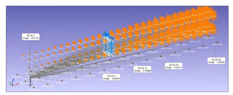
Figure 12. Uncertainty analysis of a single laser tracker station placed at the end of a 40m long cell. The increasing size of the uncertainty cloud reflects the magnitude and shape of the uncertainty measurements for that point.
