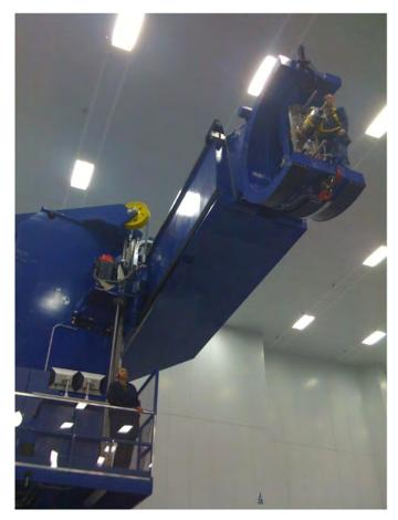
Figure 8. There is no hope of an easy reach to the toolpoint on this moving column style automated fiber placement machine with its 6.4m (21') of vertical stroke. The Active Target becomes very useful when it is time to compensate this machine.
