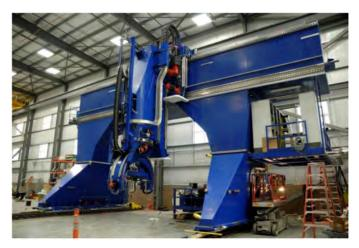
Figure 3. Gantry style automated fiber placement machine with a large working envelope. The mass of such large machines may cause significant local foundation deflections that could affect the accuracy of a laser tracker placed nearby.
