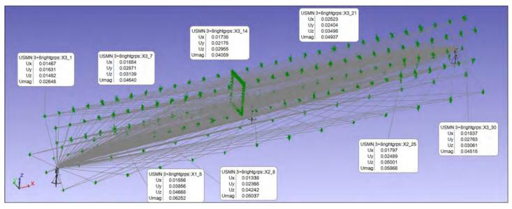
Figure 14. Uncertainty analysis of the previous cell, using 3 tracker stations. Uncertainty is now limited to about 0.07mm (. 0028") throughout the working envelope.
