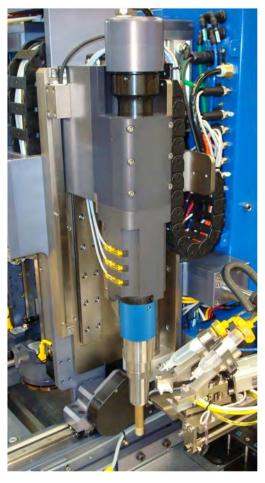
Figure 4. Bolt inserter.
