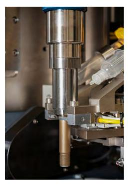
Figure 3. Sealant application.
