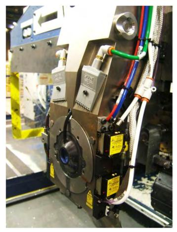
Figure 6. Headstone with laser normality sensors
