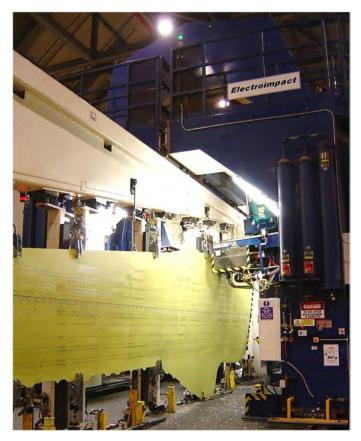
Figure 1. E4000 (SA1) machine working on an A321S panel
