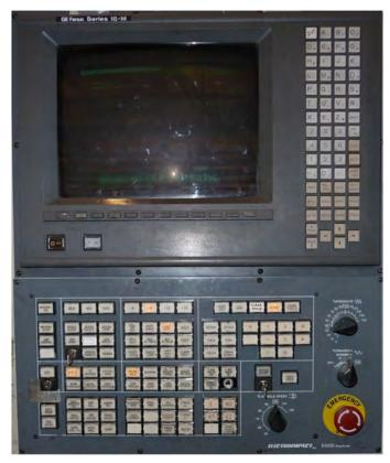
Figure 2. 15-M based operator interface
