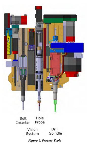
The drill spindle is driven by an 8 Newton-meter continuous rated motor and is capable of drilling holes up to 7/16 inches in diameter through carbon fiber and titanium stacks up to 1.9 inches thick. Drill feed is controlled through a servomotor and ballscrew using an absolute linear scale for secondary position feedback. Secondary feedback enables the system to have a drill and countersink feed accuracy of  $\pm$  0.0005 inches.
