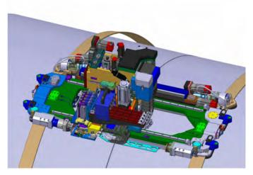
Figure 1. 5-Axis Flex Track System
