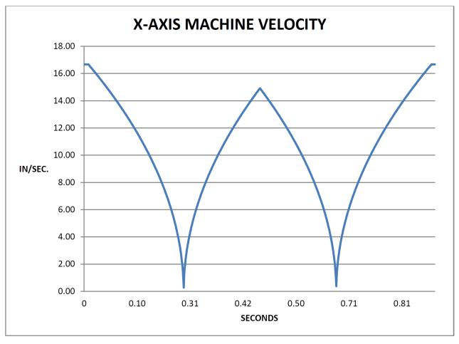
Figure 4. Machine velocity along the X-axis.
