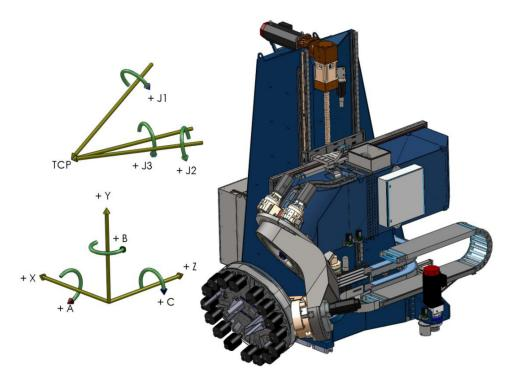
Figure 5. Naming convention for non-orthogonal axes.
