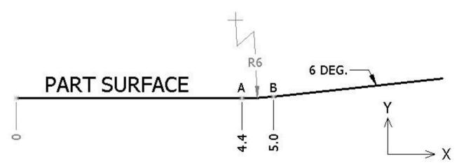
Figure 3. Small 6-degree ramp on part surface.
