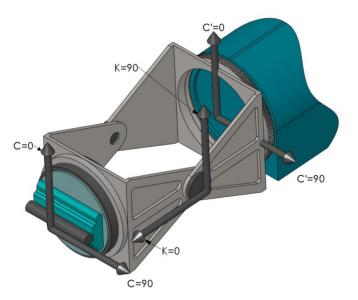
Figure 6. C'KC axis arrangement
