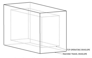
Figure 2. Machine envelope vs. Working envelope.
