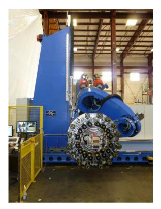
Figure 9. Electroimpact AFP machine with new rotary kinematics.
