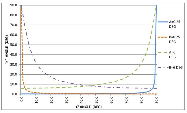
Figure 7. K and C' angles for constant A and B axis angles.
