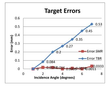
Figure 5. SMR vs Solid Prism
