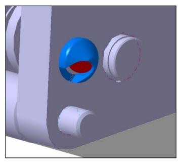
Figure 4. Laser Tracker Target Cover Concept
