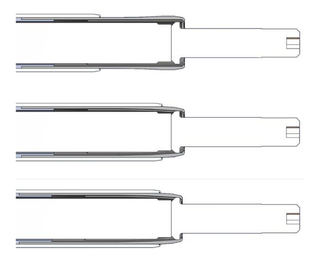
Figure 2: The three steps of loading the bolt into the collet fingers. In the third step the bolt head is pulled in registration with the pin
