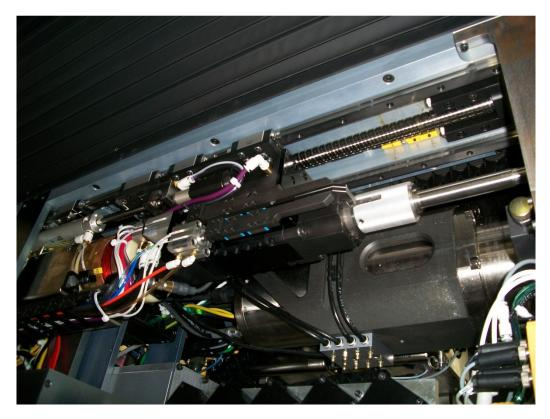
Figure 1 The EMB mounted on the riveting machine
