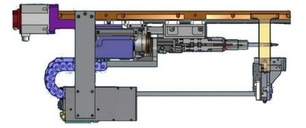
Figure 4: The end of the bolt is driven into a laser beam in order to accurately measure and confirm the bolt length before installation into the wing spar
