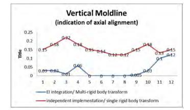
Figure 2. The above data shows the measured deviation of a mostly vertical (actually circumferential) line projected on a matching machined line on the part surface. This is an indication of the axial alignment of the laser projection to the mandrel.
