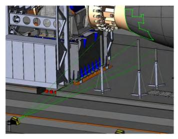
Figure 4. Laser Fiducial Stands used for locating the projector
