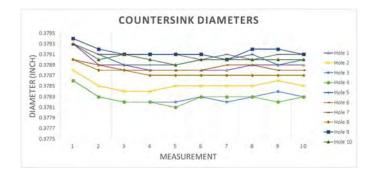
Figure 9. Series of 10 consecutive Countersink Diameter Measurements
