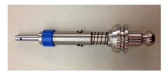
Figure 2. Typical quick-change assembly with bore gauge and countersink measurement.
