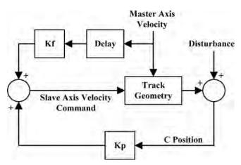
Figure 5. Block diagram of the control loop for continuous C-squaring, with feedback gain given by  $K_{p}$ .
