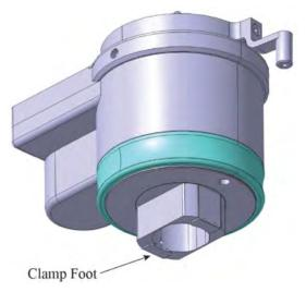
Figure 4. Nosepiece with gimbaled clamp foot.
