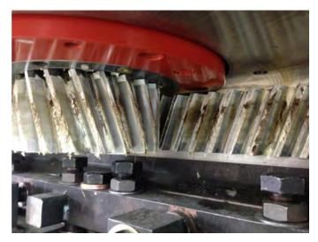
Figure 4. Rack and pinion drives require grease that must be isolated from the clean room environment.
