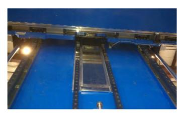
Figure 5. Attraction forces are reacted with linear rail locally around magnet plates.
