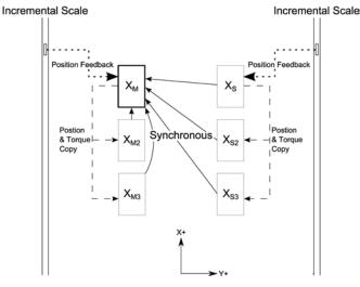
Figure 7. X-axis Controls Configuration
