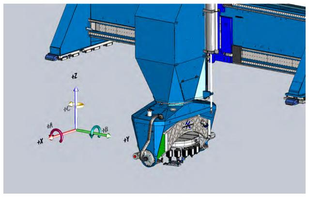
Figure 11. Machine axis coordinates.
