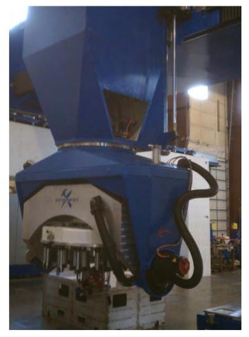
Figure 9. By utilizing a 210 degree range of motion, a Cprime axis effectively allows for 180 degrees of B-axis rotation.
