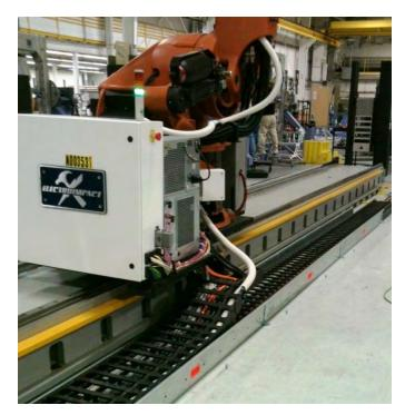
Figure 7: A Robotic Arm Mounted On a Linear Axis
