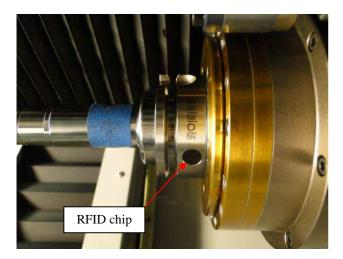
Figure 12 RFID Chip
