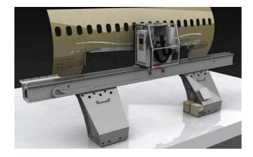
Figure 1 Side-of-Body Drilling Machine
