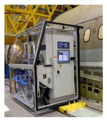
Figure 16 Side-of-Body Drilling Machine
