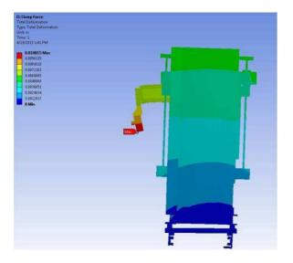
Figure 4 Machine Deflection under 1200# Clamp Force
