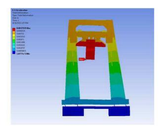
Figure 5 Machine deflection under 0.1g acceleration
