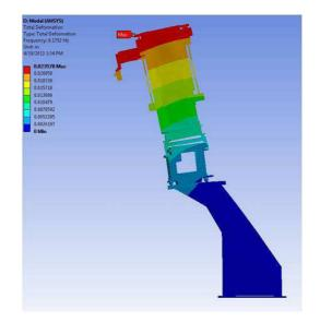
Figure 6 Modal Analysis of New Beam on Old Columns
