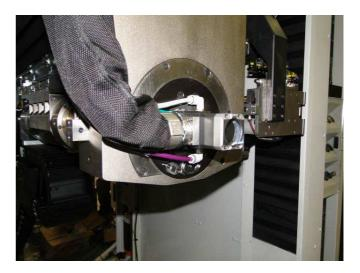
Figure 13 Pressure Foot Nosepiece
