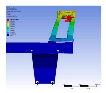
Figure 10 Machine Deflection under Shuttle Load
