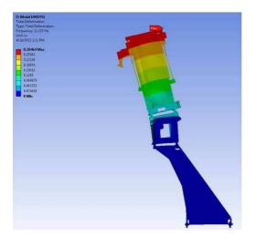
Figure 7 Modal Analysis of New Beam and Columns
