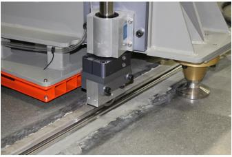
Figure 13 Air Caster and Strothmann Rail
