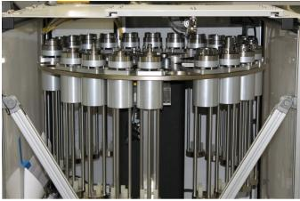
Figure 10 Automatic Tool Changer
