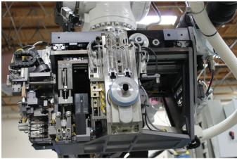
Figure 6 End Effector from Described Mobile Robot
