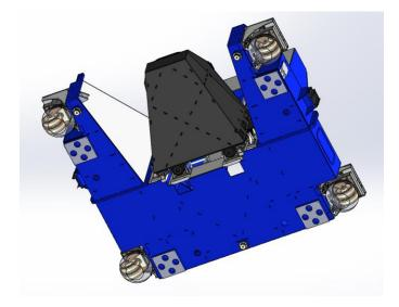
Figure 3: Bottom platform plate keeps CG low
