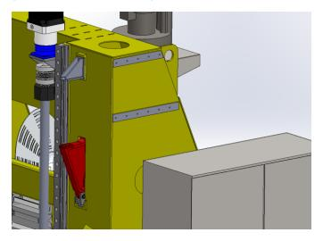
Figure 14: Hardstop/Flag indicating the Y axis is locked out; usually the Y sled would be postioned above the moving hardstop when the hardstop is extended
