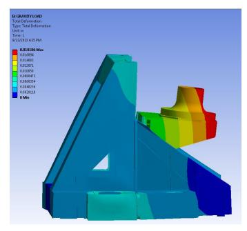
Figure 6: Sled at midpoint of stroke: overall toolpoint deflection 0.033"
