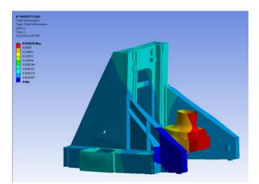
Figure 7: Sled at bottom of stroke: overall toolpoint deflection 0.033"
