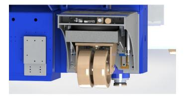
Figure 10: pneumatically deployed caster with rigid mount swivel foot in background
