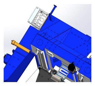
Figure 2: Tower structure with increased section and plate backing up vertical rail
