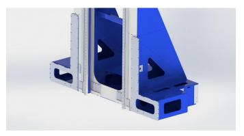
Figure 12: Side bolster and platform deck are designed to be a structural plinth and mounting surface, with good access from top and sides
