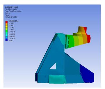
Figure 8: The Y sled was analyzed as part of the system with the frame and the robot base
