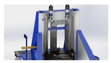
Figure 9: Dual Heidenhain absolute glass scales, mounted outboard of the Y rails
