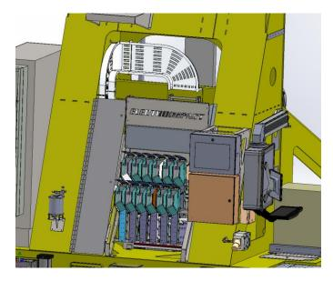
Figure 11: Routing of wireway allows freedom to place equipment, and access to equipment from both sides when it is in place
