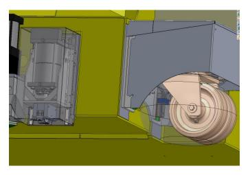
Figure 13: Pneumatically deployed Strothmann wheel for rail guidance, mounted near lifting caster
