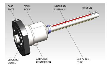
Figure 3. Lower tubular clamp inside riveting anvil.
