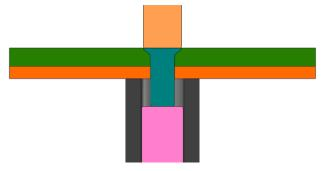
Figure 2. Schematic of normal rivet installation
