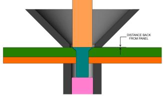
Figure 10. Upper anvil slightly retracted and DISTANCE BACK FROM PANEL..
