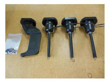
Figure 4. Range of lower anvil tooling.
