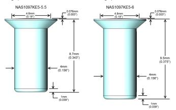
Figure 1. NAS1097KE5 rivets with dimensions. Page 1 of 4
