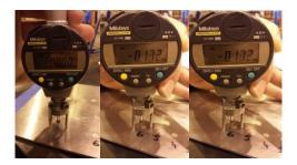
Figure 6. Measurements showing dimpling in stacks thinner than 4mm.
