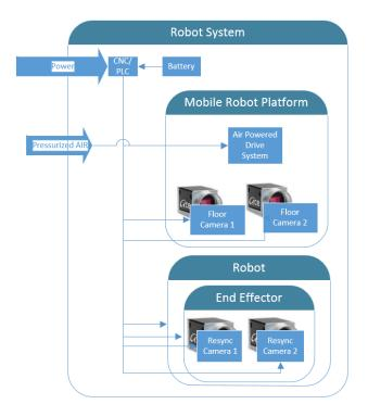
Figure 2 System Architecture
