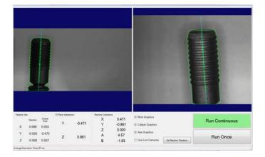
Figure 11 3D Vision of Fastener Tails
