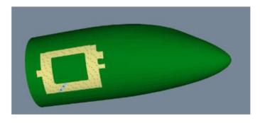
Figure 5. Operator display highlights course laser is projecting
