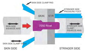
Figure 3. Rivet insertion and seating in the countersink.
