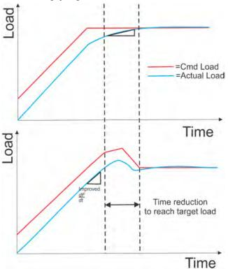
Figure 12. Showing a zoomed in view of the upset load profile at the transition from ramp to dwell. The first image shows a standard transition, while the second shows the improved performance by adding artificial overshoot.
