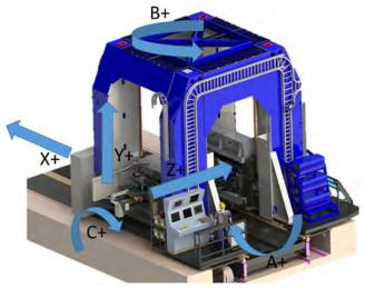
Figure 1. Vertical fastening machine overall arrangement.
