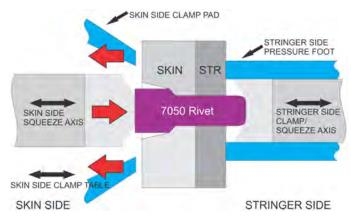
Figure 4. During the Servo/Servo move, the head is pinned into the countersink by the squeeze axis.
