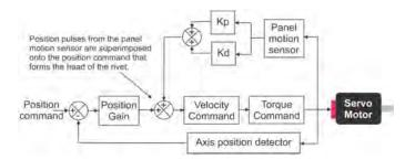
Figure 8. Skin side forming axis process control loop.
