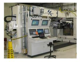
Figure 7 PAL test bench includes the operator control, process tools, shuttle table, clamp tables and vacuum system of actual production machine.
