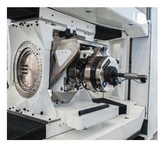
Figure 13 Rivet forming process head, V-side.
