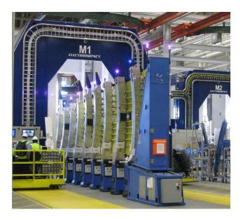
Figure 14 Machine and Tools use the same base structure to maintain alignment and reduce differential movement.
