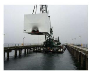
Figure 11 the barge crane with machine suspended moving away from the loading area to transfer the machine to the transport barge.
