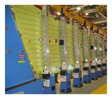
Figure 16 Tooling posts were placed in complementary positions from one cell to the next to avoid manipulating the tool during production.
