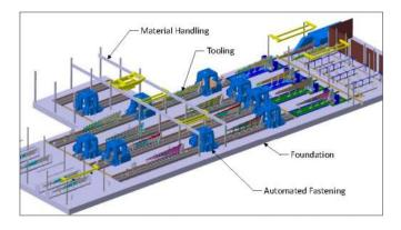
Figure 2 Panel Assembly Line (PAL) Subsystems.
