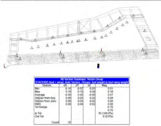
Figure 12. Spatial Analyzer results for the live load of loading the wing into the fixture (rear spar (top beam) weights only)
