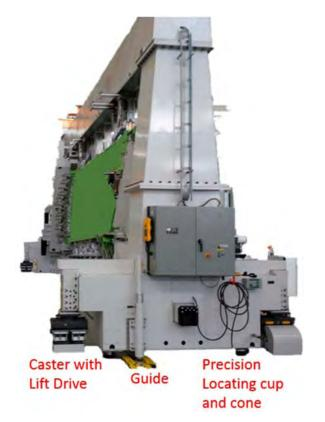
Figure 1. Alternative caster-supported system considered
