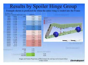
Figure 9. Example of Deflection Predictions for a Live Load
