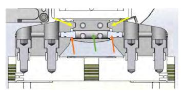
Figure 11. M20 EOAT gripper finger wedge and backup pin cross-section.
