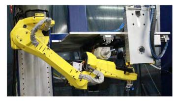
Figure 17. M10 robot in position for a close clearance pick on ATC testbench.
