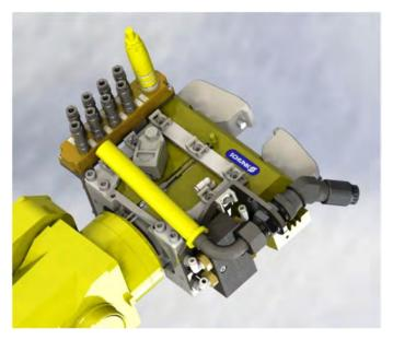
Figure 10. M20 robot EOAT
