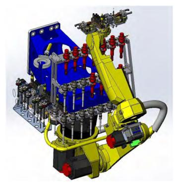
Figure 5. M10 robot with tool rack containing drill bits, hole probes and bolting anvils.
