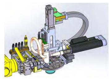
Figure 4. 3/8" nutrunner nosepiece in M20 EOAT
