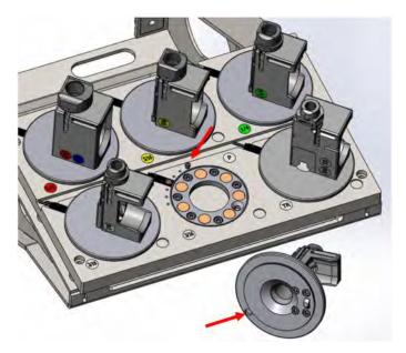
Figure 16. Vacuum nosepiece tool identification. Each nosepiece has a unique counterbore pattern which mates with a unique pin pattern on the rack (red arrows).
