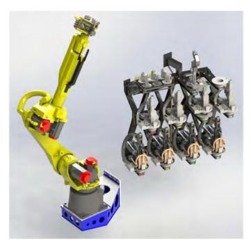
Figure 8. M20 robot with nosepiece rack.
