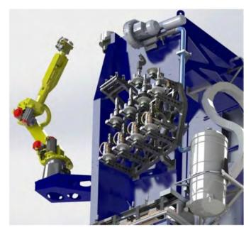
Figure 13. Nosepiece rack on side of machine tower. Note the structural wall between robot and rack.
