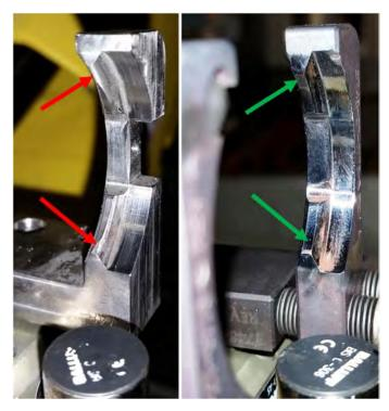
Figure 18. Wear on M10 EOAT gripper fingers after several hundred thousand cycles (at left). Compare this to a brand new set of fingers (right).
