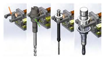
Figure 2. M10 EOAT in various states. Left to right: empty, gripping drill bit, gripping hole probe, gripping bolting anvil. Note all tools mate with the same gripper locating taper (orange arrow) and clocking dowel (green arrow).
