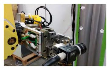
Figure 19. Robotic Vision testing using a camera held in the M10 EOAT sighting three targets.
