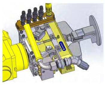
Figure 3. 3/16" vacuum nosepiece in M20 EOAT
