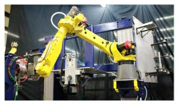
Figure 9. M20 robot at machine socket during a nosepiece tool pickup.
