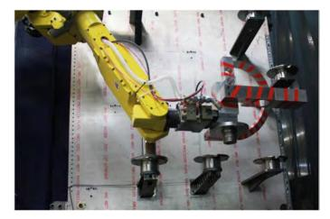
Figure 14. M20 robot reaching to the collar swage / nutrunner / vacuum nosepiece tool rack during high payload testing.
