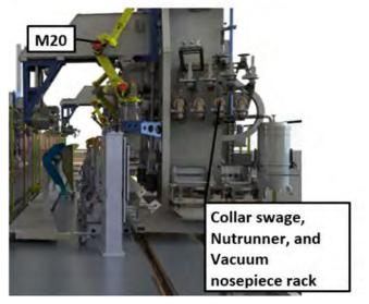
Figure 1. Machine front/side views showing locations of ATC components. These include M10/M20 robots, tool storage racks, and the machine sockets/ shuttle table housing in-use tools.
