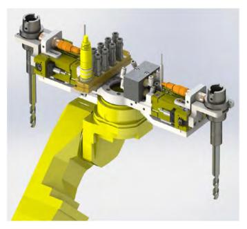
Figure 7. M10 robot EOAT
