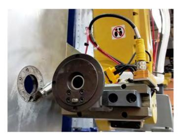
Figure 12. The M20 EOAT cleans a machine tool socket immediately prior to installing the vacuum nosepiece.
