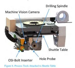
Located behind the nosepiece is load cell that is used to ensure the end effort is being pushed up to the work piece at the pre-defined load. The end effector also contains all of the process tools, such as the drilling spindle, hole probe, machine vision camera and the OSI-Bolt inserter. These process tools are all mounted to a shuttle table, as shown in <u>Figure 6</u>, so that the entire process can be performed without having to reposition the end effector.
