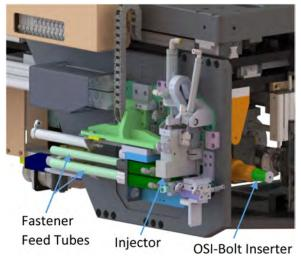
Figure 12. Fastener Injector on Side of End Effector
