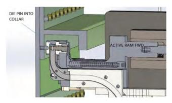
Collar Cycle Step 4. Die pin extended into collar
