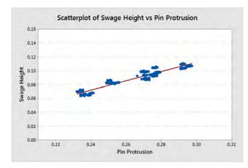
Figure 12. Collar Swage Height vs. Bolt Pin Protrusion
