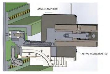
Collar Cycle Step 1. Anvil clamp up, active ram retracted
