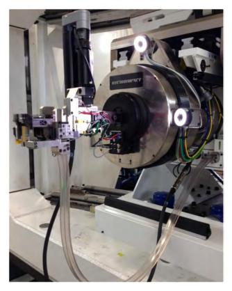
Figure 6. Nut runner anvil installed on PAL machine at Electroimpact
