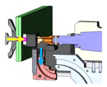
Nut Cycle Step 4. Socket strips fastener from loader fingers as loader retracts. Hi-Lok is inserted and rod lock is released.
