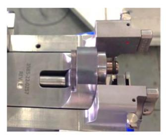
Figure 9. Offset collar tool with active ram retracted
