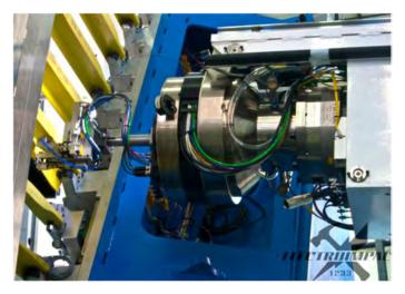
Figure 2. PAL machine navigating 737 stringer with offset tool installed at Electroimpact
