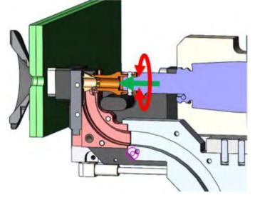
Nut Cycle Step 3. Machine drives forward while spindle performs amble routine, engaging 12-point pattern with socket and retaining spring. Rod lock is actuated while bolt is fed.
