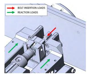
Figure 10. Bolt insertion reaction loads
