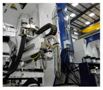
Figure 4. LGP collar and TN nut feed path shown with buffers and vibratory bowls
