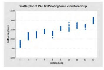
Figure 11. Bolt Seating Force vs. Installed Grip
