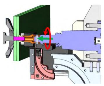
Nut Cycle Step 5. Spindle runs nut down Hi-Lok threads and torques to specification. Machine unclamps.
