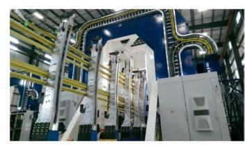
Figure 1. Wing fastening system running with parallel gripper injector
