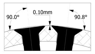
Figure 5. Fastener head protrusion caused by off-normal drilling and countersinking. Shown are 3/16" flat head fasteners on a curved panel with 45mm bend radius.
