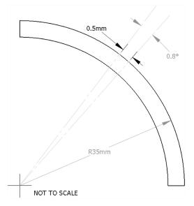
Figure 4. On a highly curved surface, a positional change of 0.5mm can change the angle of the normal vector by 0.8 degrees.
