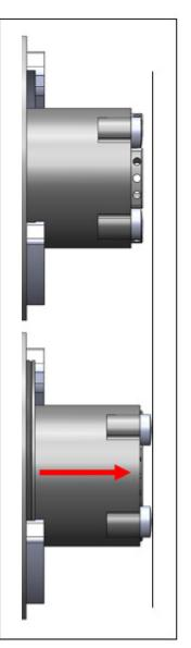
Figure 7. Compressed air is used to extend the spherical pads forward of the base contact surface. The actuated lander is shown in the retracted position, upper, and extended position, lower.
