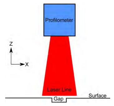
Figure 2. Profilometer Diagram
