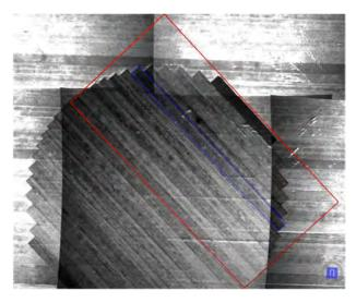
Figure 10. Ply Image with Highlighted Course and Tow.
