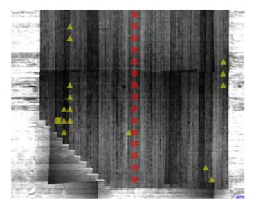
Figure 12. Lap Gap Errors Overlaid on 3D Model of Ply.
