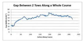
Figure 7. Gap width measured every 0.5" along course direction.
