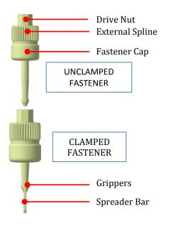
**Figure 3: Key Fastener Features**
