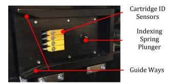
Figure 5: Cartridge Receiver Assembly
