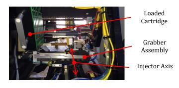
Figure 7: Injector Assembly Components
