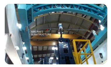
Figure 5. Extended lower ram hitting substructure
