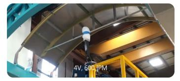
Figure 13. Lower ram hitting part structure during testing
