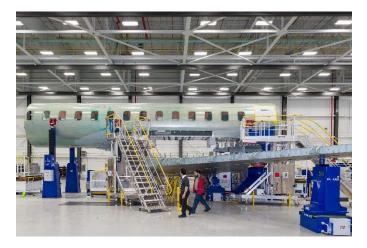
Figure 4 Wing to fuselage join laser trackers are hidden behind surrounding equipment. Photo credit: Robert Backus.
