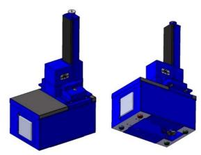
Figure 12: Single positioner module of the APS. Foundation cup/cone interface (right).
