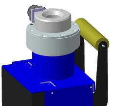
Figure 13: Custom handling ball receiver. Lateral float with lockout. Ball sensing and retaining. Spring actuated and pneumatically released in a tight package.
