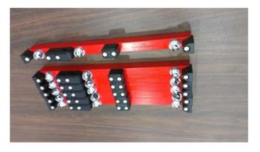
Figure 18 Vector bars used for aft fuselage joins.
