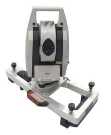
*Figure 19 A custom stand is used to mount the tracker on the a/c seat track rails.*
