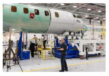
Figure 5 Forward fuselage join is achieved via feedback from tracker mounted inside the fuselage. Photo credit: Robert Backus.
