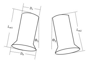
Figure 4. Fastener Measurements In Single Image
