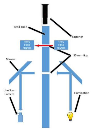
Figure 3. Inspection Method Geometry
