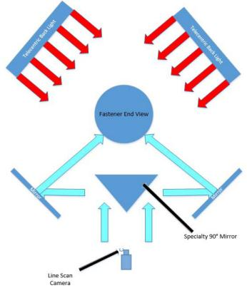
Figure 2. Optical Inspection Layout
