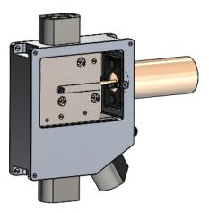
Figure 7. Fastener Eject Actuator Assembly
