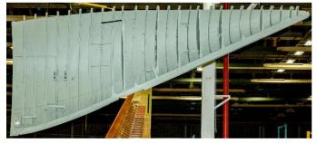
Figure 3. Right side panel of C-130J aft fuselage with structure visible, showing deep circumferential frames that must be fastened directly to the skin.
