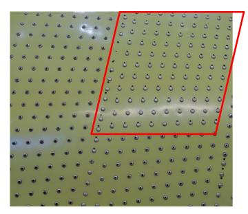
Figure 10. This example of an array of fasteners show areas that needed adjustment (in red) and fastener locations that were correct found during pen plotting.
