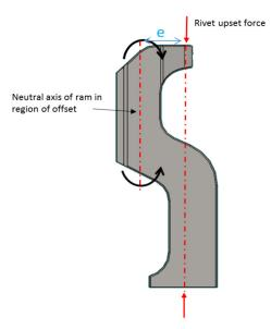
Figure 4. Illustration of internal bending moment applied to offset riveting anvil ram.
