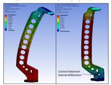
Figure 5. Comparison of lateral deflection in conventional offset anvil ram versus ram with optimized cutout.
