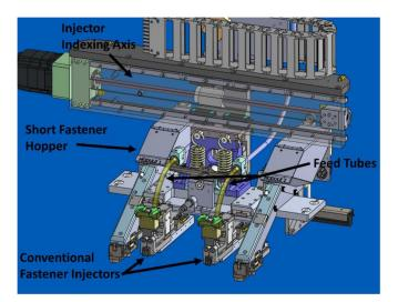
Figure 7. Injector array showing combined hoppers and fastener injectors.
