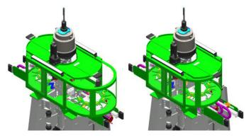
Figure 8. ATC enclosure (depicted here in green), fully encapsulates anvils.
