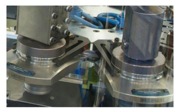
Figure 4. ATC grippers and tool interface
