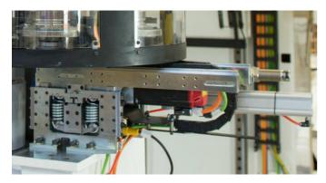
Figure 7. Preloaded springs allowing for vertical compliance
