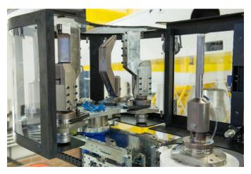
Figure 5. Crescent shaped carousel and fastening head (carousel shown in expanded position)
