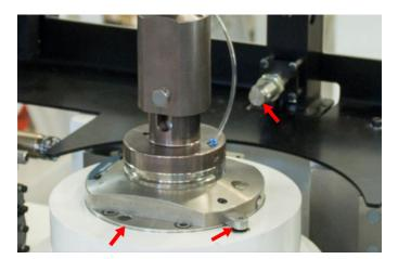
Figure 8. Left to right: Machine interface, tool RFID chip, and air nozzle
