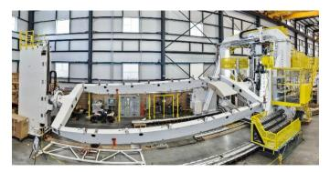
Figure 1. Electroimpact Skin Splice Riveter.
