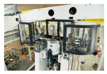
Figure 3. ATC and lower fastening head below test panel
