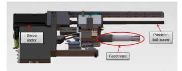
Figure 4. Servo-driven bolt inserter
