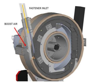
Figure 10. Fastener and airflow inlet.
