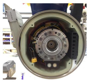
Figure 6. Partially disassembled rotor with plastic components.
