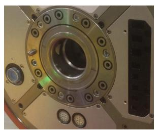
Figure 8. Automatic tool changer interface.
