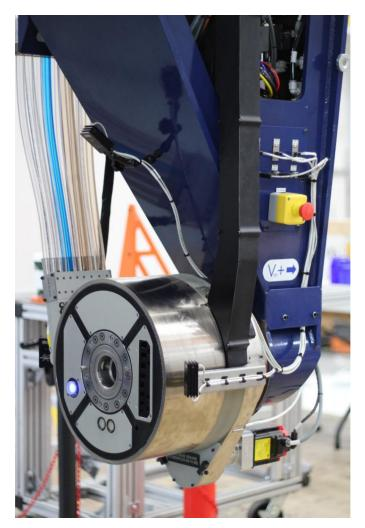
Figure 3. C Axis with spinner assembly.
