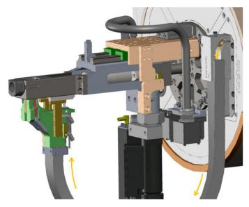
Figure 14. Fastener received by anvil and conveyed to tool point.
