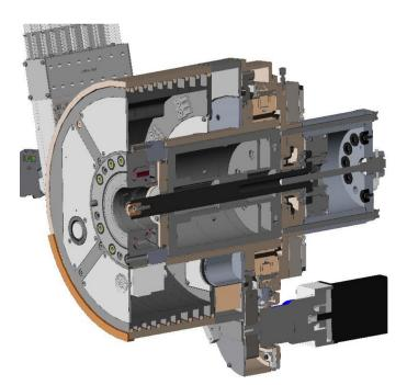
Figure 9. Spinner cutaway with rotor/stator configuration shown.
