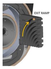
Figure 13. Fastener exiting spinner.
