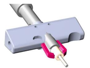
Figure 10. EMR fingers stripped back over the die
