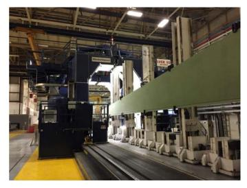
Figure 13. LVER machine with wing panel
