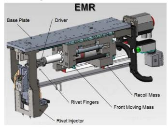
Figure 3. Electromagnetic riveter retracted
