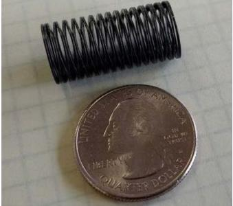
Figure 11. Wave spring pushes fingers closed
