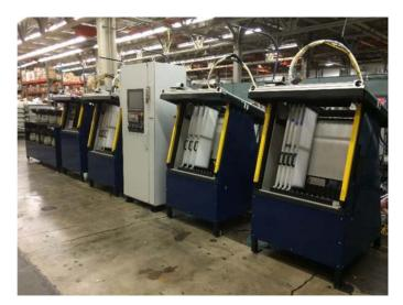
Figure 2. Off-Line Cartridge Filling Station
