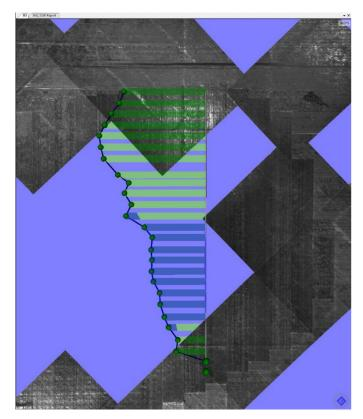
Figure 7. Overlap/Gap Errors Overlaid on 3D Model of Ply.
