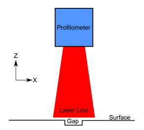
Figure 2. Profilometer Diagram
