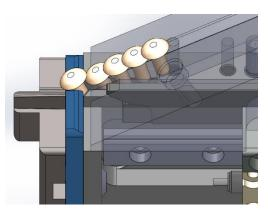
Figure 12: Example of rivets jamming in conventional mini-hoppers
