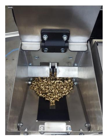
Figure 9: Flexible riveter hopper
