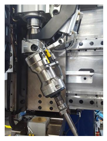
Figure 6: Rivet ram and automatic drawbar
