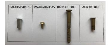
Figure 15: Wide variety of parts flexible riveter can feed
