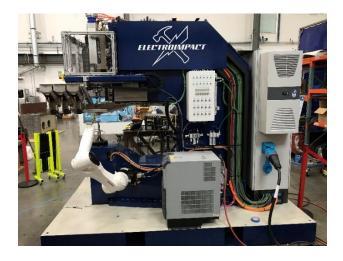
Figure 2: Flexible all electric riveter
