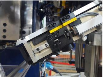
Figure 11: Air cylinder injecting rivet
