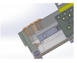
Figure 13: Flexible riveter feeding unjammed rivets
