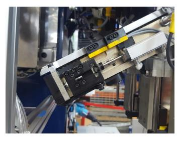
Figure 10: Air cylinder separating rivet
