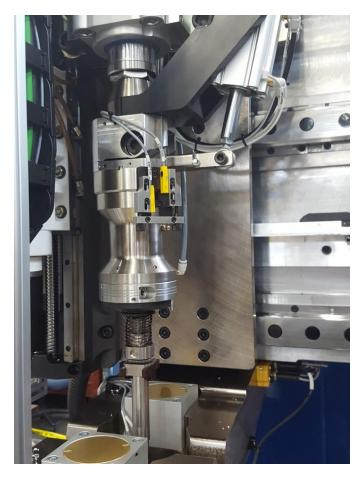
Figure 5: Rivet ram, automatic drawbar and zero clamp
