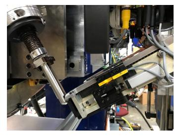
Figure 4: Air cylinder mechanism in contact with the hopper
