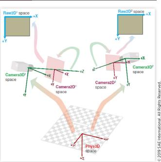
squared error function is minimized using gradient decent to solve for the 12 linear parameters. This calculation is common in machine vision software and its results are not investigated here. What these parameters define are important to understanding how this 3D stereo vision functions.
