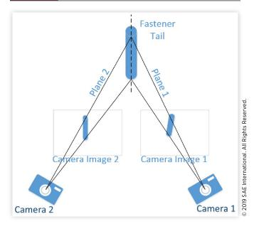
parameter. This is done for both cameras to create two intersecting planes (<u>Figure 8</u>). The location at which these planes intersect is the centerline of the fastener in 3D space.
