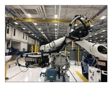
Figure 4. Processing a small component – in this case a fairing
