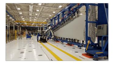
Figure 5. Robot system working on a rudder which is one of the larger assemblies processed by the automation
