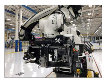
Figure 1. Electroimpact MFEE coupled with Accurate Robot.
