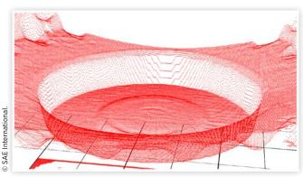
**FIGURE 7** Example of the "knee" inflection points located at the inner diameter of the nosepiece.
