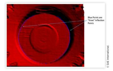
Custom method "FindKnees" is run to determine inflection points of a specific angle and intensity that could be the edge of the nosepiece. The filtering criteria has been adjusted to specifically find edges similar to the nosepiece geometry.
