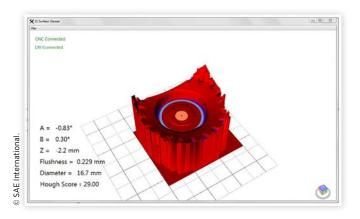
The diameter of the nosepiece is used to cross check that the correct tooling has been installed. The A, B, and Z are used to determine and correct the machine orientation in relation to the panel. The flushness is relayed to the operator and checked to ensure it is within tolerance. And finally the Hough Score is not entirely necessary for the operator, but it gives an example of the circle strength and possible need to clean the nosepiece or the laser.
