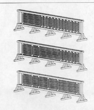
THE OPERATOR REMOVES THE FIRST SEVERAL FORMBOARDS TO OPEN UP A BAY. THE AERAC INSTALLS RIVETS DNE ONE SIDE OF THE ALL STRINGERS BEFORE THE OFFSET TOOLING IS ROTATED AND RIVETS ARE INSTALLED ON THE OPPOSITE SIDE OF THE STRINGERS. THE END FORMBOARDS ARE NOT REMOVED ON THE AERAC SINCE THEY DO NOT OBSTRUCT ACCESS TO ANY RIVETS.
