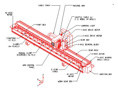
Figure 2. - The Automatic Stringer Drilling System
