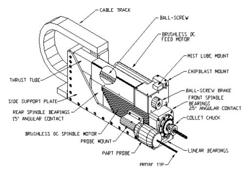
Figure 3. - Model 04 Servo-Servo Drill
